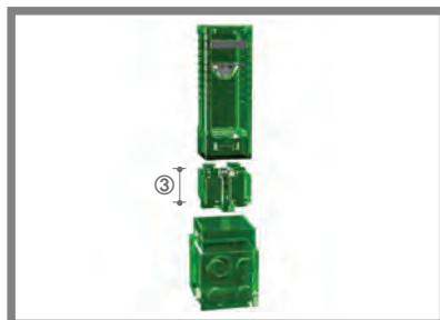
Separate fixture ampule from bottom, as shown, to reveal cover screw holder ®
